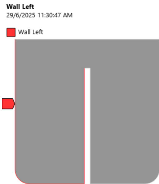
Figure 4. Wall left boundary condition setup with Temperature , T = 80\text{ }^{\circ}\text{C}
